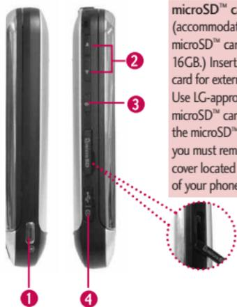
microSD™ card slot (accommodates optional microSD™ card up to 16GB.) Insert microSD™ card for external memory. Use LG-approved microSD™ card. To access the microSD™ card slot you must remove the side cover located on the side of your phone.
